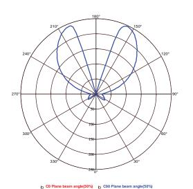
C0 Plane beam angle(50%):80.0(DEG) C90 Plane beam angle(50%):324.2(DEG)
