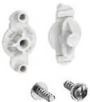
Fixing element for mounting of enclosure on cable tray systems with elongated hole width of 7 mm and mesh cable trays with Schnabl GTH 9001 mounts. With pan head screw 4 x 12, material PA6 grey, Set = 10 pieces
