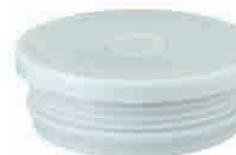
Sealing plugs, IP55, with closed sealing membrane, thermoplastic elastomer (TPE), for wall thickness 1.5 - 4.0 mm, for sealing of metric housing apertures that are not required, grey
