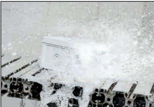
**Water and contact protection testing**
