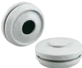
Double membrane seals, IP66, with two sealing membranes, closed, thermoplastic elastomer (TPE), for wall thicknesses 1.5 - 4.5 mm, grey
