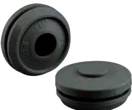
Double membrane seals, IP66, with two sealing membranes, closed, thermoplastic elastomer (TPE), for wall thicknesses 1.5 - 4.5 mm, black
