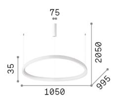
Net weight3.1 kgInsulation classIProtection indexIP20ComplianceCEOperating temperature $0^{\circ} \sim +40 \, ^{\circ}\text{C}$
