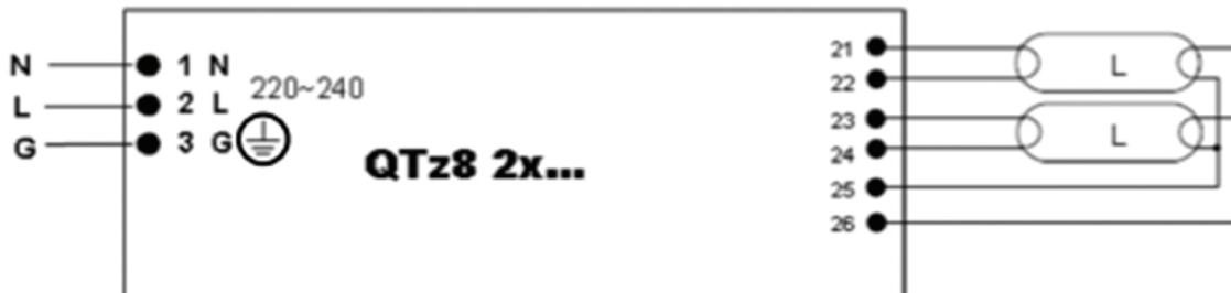
Max. permitted cable length in between ECG and lamp: 1.0 m (PIN 21, 22, 23, 24); 2.0 m (PIN 25, 26)
