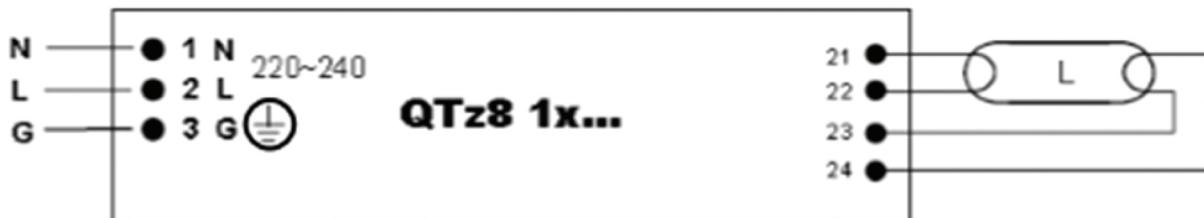
Max. permitted cable length in between ECG and lamp: 1.0 m (PIN 21, 22); 2.0 m (PIN 23, 24)
