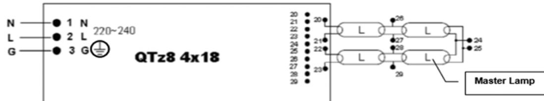
Max. Permitted cable length in between ECG and lamp: 1.0 m (PIN 20, 21, 22, 23); 2.0 m (PIN 24, 25, 26, 27, 28, 29)
