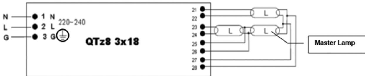
Max. Permitted cable length in between ECG and lamp: 1.0 m (PIN 21, 22, 23, 24); 2.0 m (PIN 25, 26, 27, 28)
